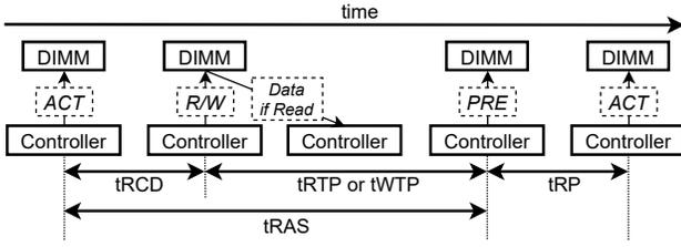
Figure 1: DDR3 Timing Parameters
