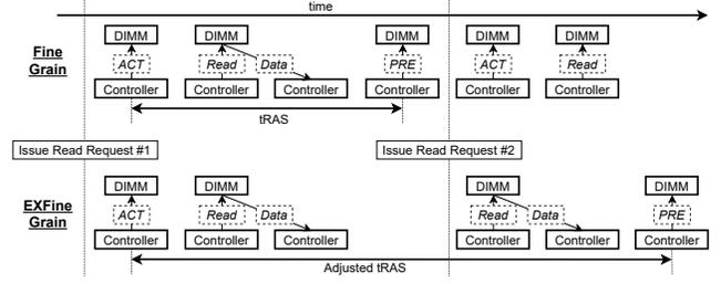
Figure 2: Behavior Comparison of the Fine-Grain Model and the Extended Fine-Grain Model
