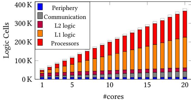
**Figure 8.** Resource Utilization for different core counts. Note that the data in L1 and L2 caches is not stored in logic cells but special memory not included in this figure.
