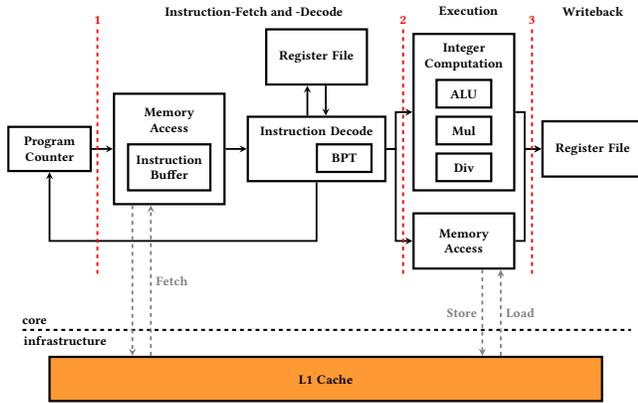
**Figure 3.** Structure of the pipelined processor with in-order execution.
