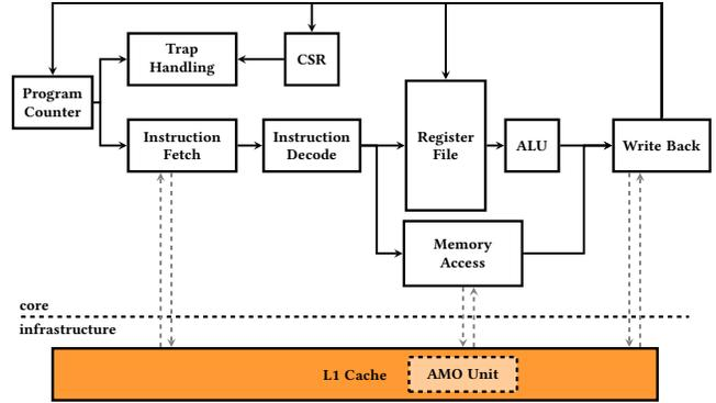
Figure 6. Structure of the size-optimized processor core with basic support for parallel programming
