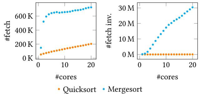
Figure 7. L2-Cache statistics for fetches (left side) and invalidating fetches (right side)
