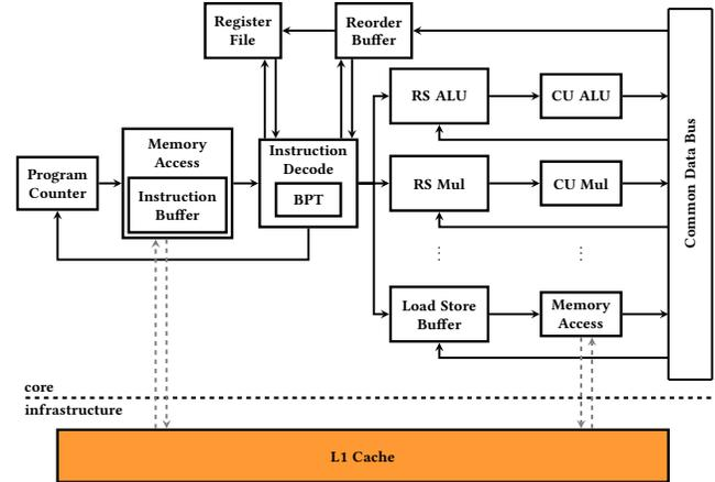
**Figure 4.** Structure of the pipelined processor with out-of-order execution (pipeline stages are not shown here).
