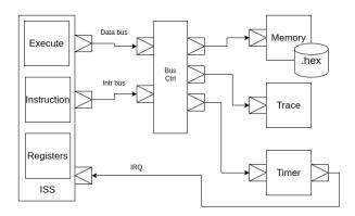
Figure 1: TLM Diagram of the entire simulator
